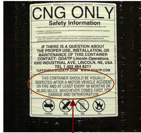
Figure 6: CNG cylinder label with inspection requirements (11)
